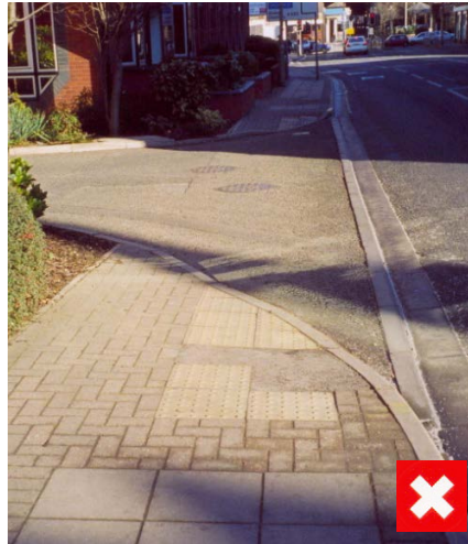
Large corner radii allows drivers to turn without slowing very much
