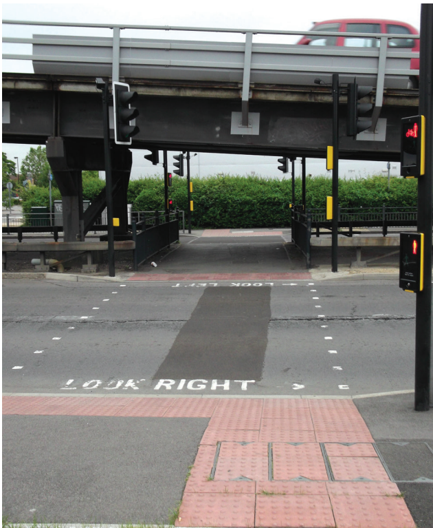
Two-stage nonstaggered toucan crossing with nearside aspects to prevent "see through"
