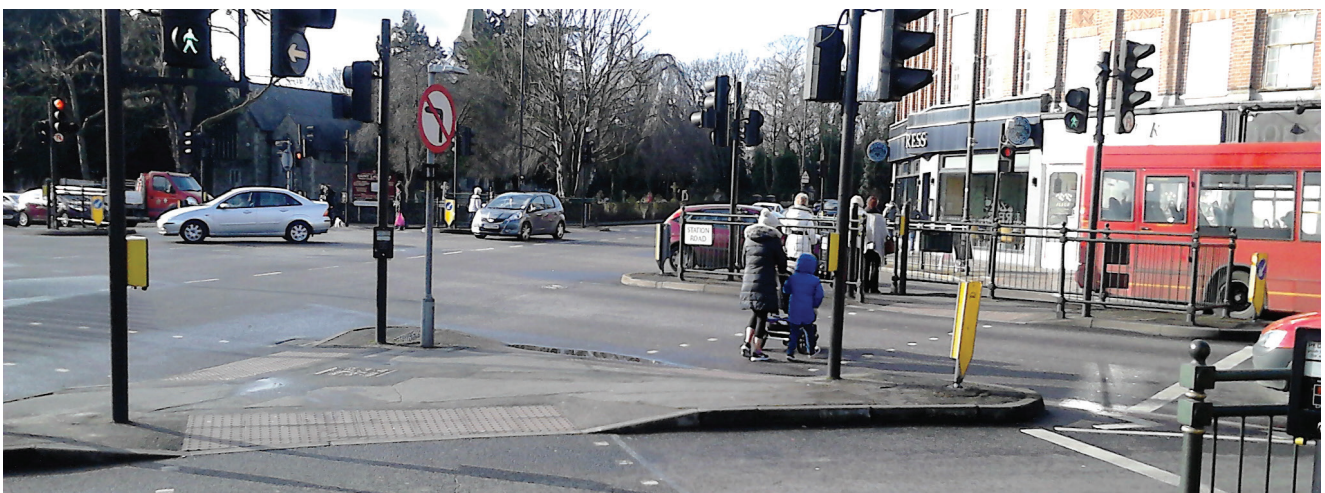
Multistage crossing at a junction
